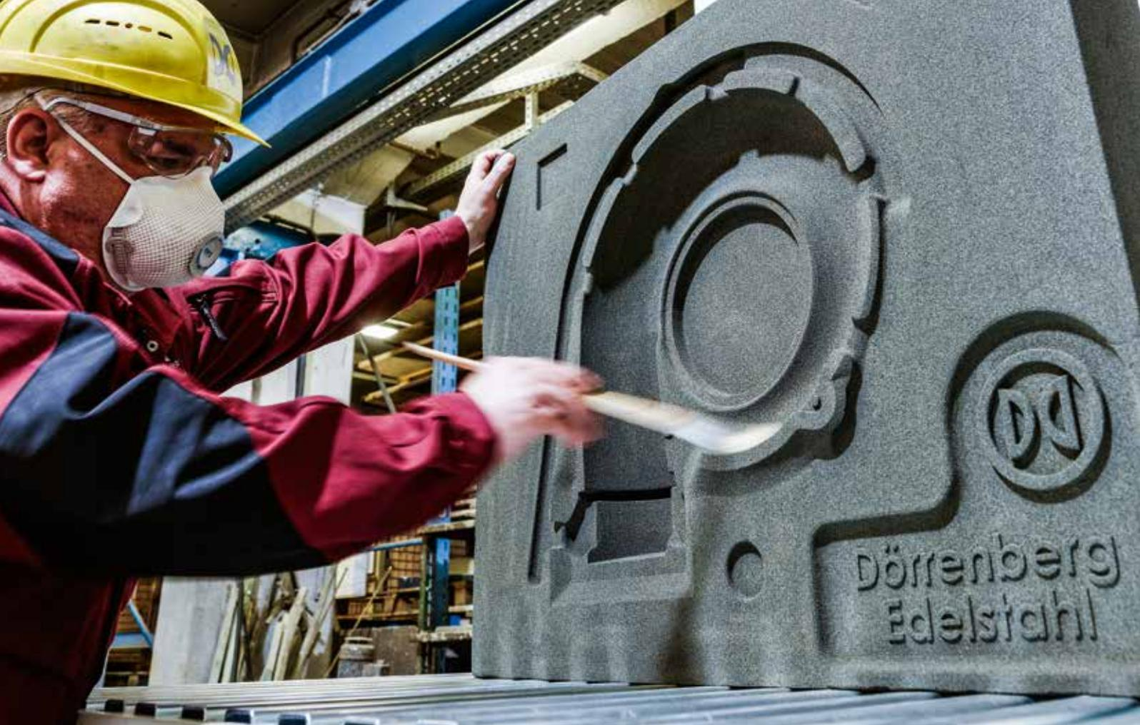
A printed sand mould is cleaned of excess sand
