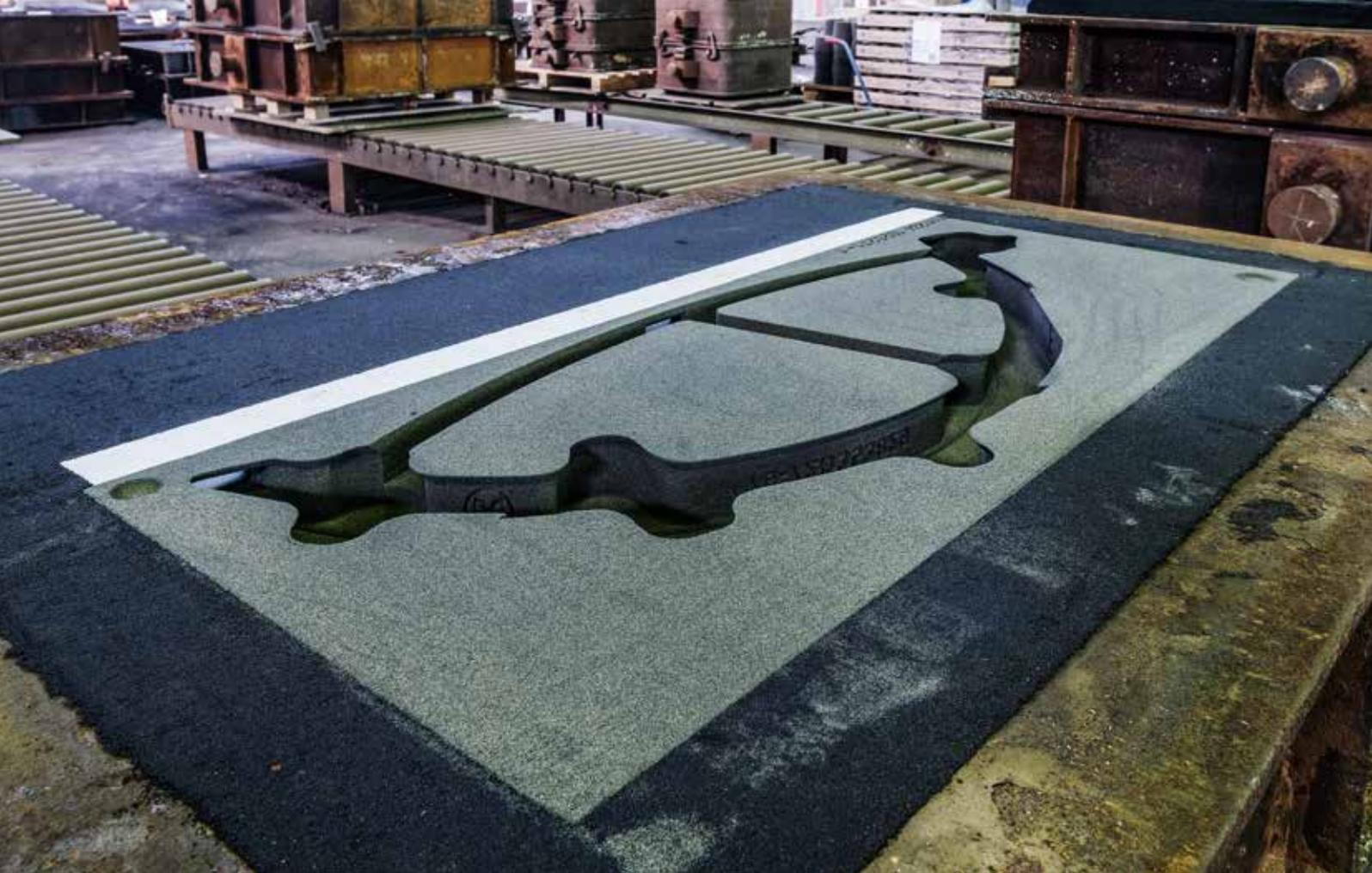
*Divided printed sand moulds are embedded in moulding sand*
